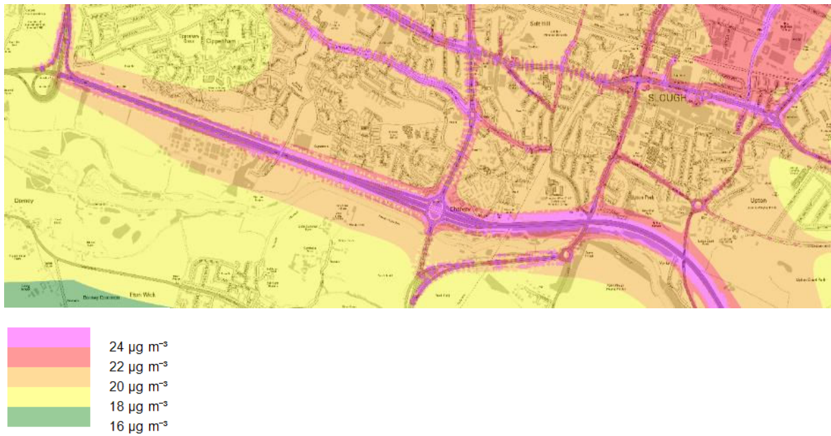
Figure 6 - Modelled PM2.5 concentrations for 2014 in the Town Centre, at Tuns Lane and along the M4
